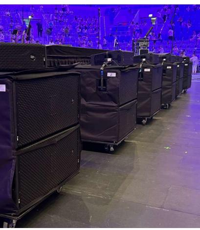
The cardioid configuration of LARA and LARA SUB enabled rear attenuation of up to -15 dB in low frequencies, significantly reducing unwanted sound at the back of the stage. Moreover, an advanced choral microphone setup was designed with multiple lines and directional systems, ensuring that each voice was naturally captured and blended into the mix.
